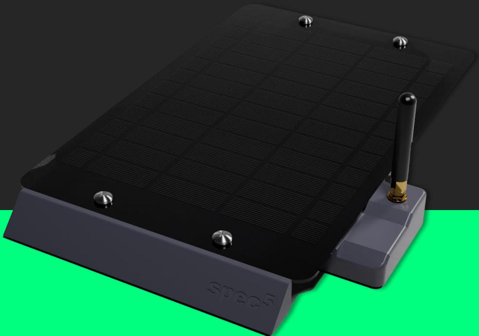
**WARNING: ALWAYS ATTACH THE INCLUDED ANTENNA BEFORE POWERING ON THE SPECFIVE VOYAGER. POWERING IT ON WITHOUT THE ANTENNA CAN CAUSE PERMANENT DAMAGE TO THE DEVICE.**
