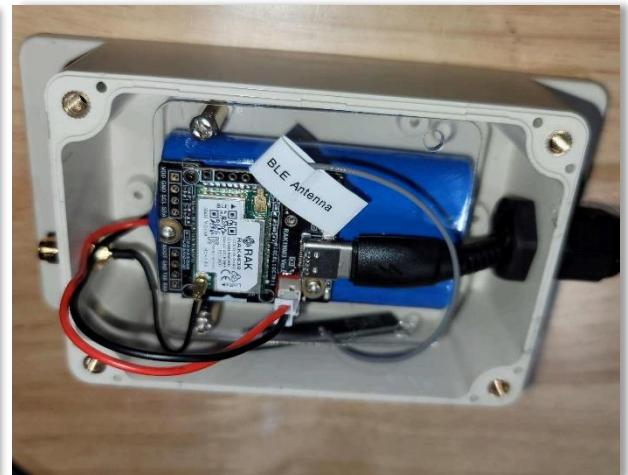
Once the battery is connected the SpecFive Relay will be powered on as there is no power switch. Please be mindful that the battery will drain when it is connected to the board without 5 volt Power input from the USB, either from an external power source or the provided Solar panel.
